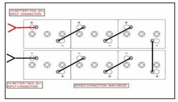
Figure 12: The batteries connected in series.
