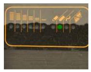
Figure 4: The LED display on top of the charger indicates when the battery is completely charged. For a complete list of LED messages, see page 17.
