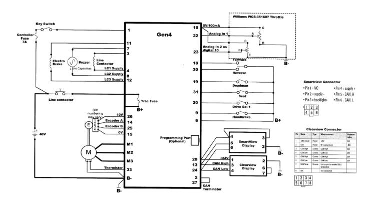
Figure 17: Typical Controller wiring configuration.
