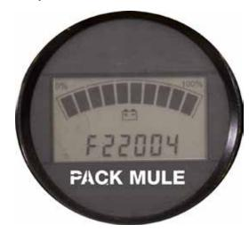
Figure 18: The Smart View display indicating a fault.
