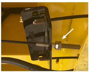
Figure 14: To adjust the mechanical drum brakes, advance the two nuts on the central rod (indicated by the arrow).
