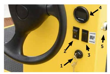
Figure 5: The instrument panel showing (1) the key switch, (2) the rocker on/off switch, (3) the directional selector switch, (4) the Smart View display, and (5) the horn button..
