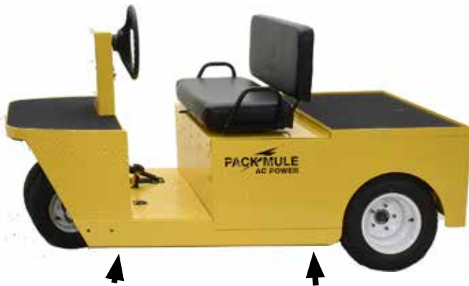
Figure 13: Position the jacks or jack stands
