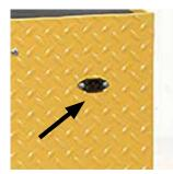
Figure 3: The charging receptacle is located on the upper right side of the rear panel. The cord is stored beneath the cargo deck.
