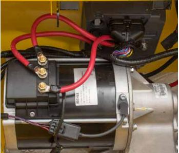
Figure 15: The motor connected to the Sevcon motor controller.
