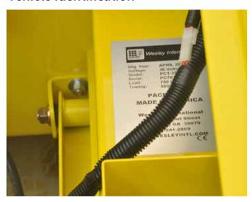
Figure 2: The Vehicle Identification Plate is located on the inside of the motor compartment. Please refer to this information when requesting warranty service, ordering replacement parts, or requesting service support from Wesley International.
