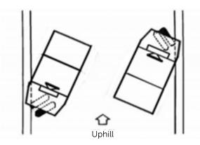
Figure 8 Proper positioning of the Pack Mule's front wheels when parking on an incline.
