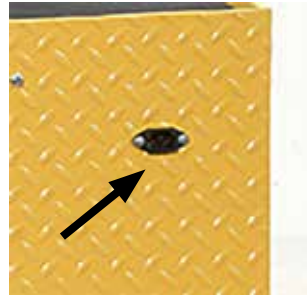
Figure 3: The charging receptacle is located on the upper right side of the rear panel. The cord is stored beneath the cargo deck.
