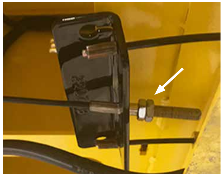
Figure 14: To adjust the mechanical drum brakes, advance the two nuts on the central rod (indicated by the arrow)..
