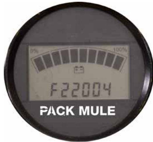
Figure 18: The Smart View display indicating a fault.
