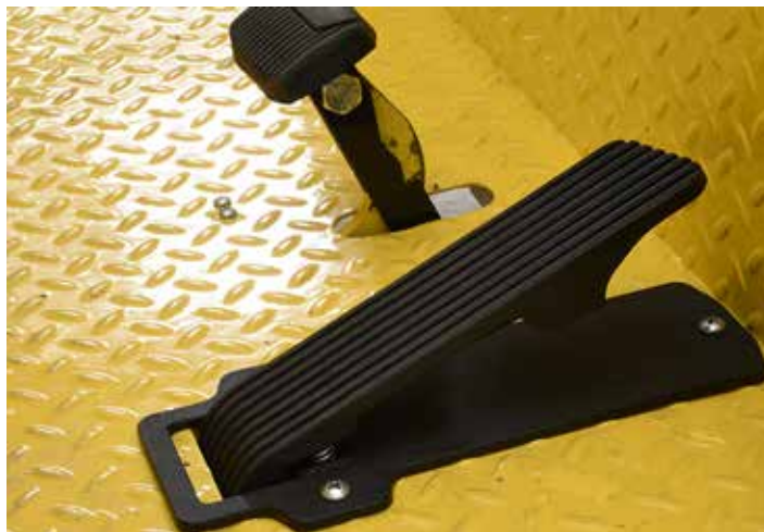
Figure 7: The Accelerator/Brake Pedal. With the key switch turned to "On", and the directional switch at "Forward" or "Reverse", the pedal puts the vehicle in motion. When the pedal is released, the vehicle stops. .
