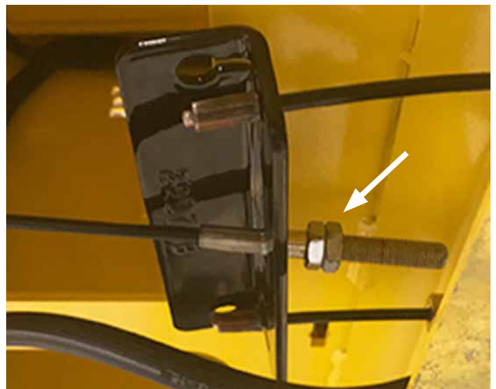
Figure 13: To adjust the mechanical drum brakes, advance the two nuts on the central rod (indicated by the arrow)..
