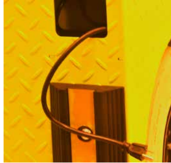
Figure 3: The AC cord for charging the batteries. Simply extend the cord and plug it in to an appropriate receptacle.
