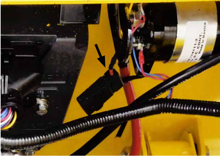
Figure 9: The fuse (indicated by the arrow) should be removed before performing any maintenance or repair work on the electrical system.
