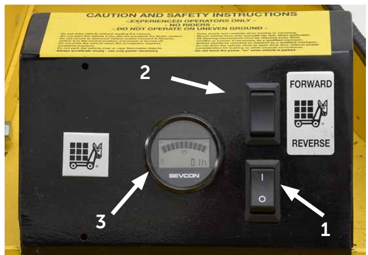
Figure 5: The instrument panel showing (1) the on/off switch, (2) the directional selector switch, and (3) the Smart View display.
