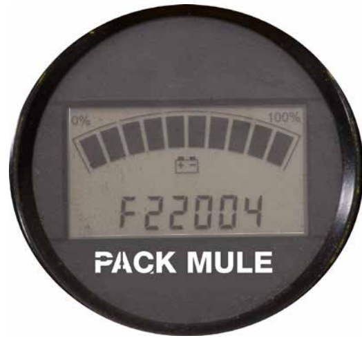
Figure 15: The Smart View display indicating a fault.
