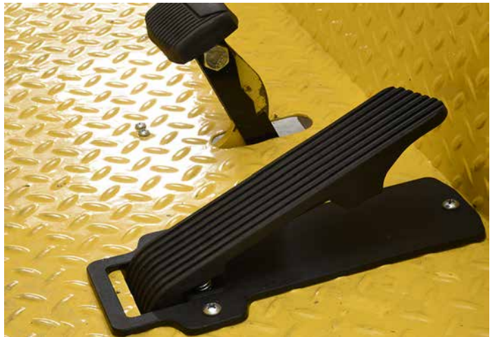
Figure 7: The Accelerator/Brake Pedal. With the key switch turned to "On", and the directional switch at "Forward" or "Reverse", the pedal puts the vehicle in motion.
