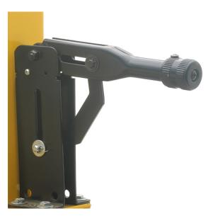
Figure 7: The optional parking brake in the OFF position. Parking brake tension may be adjusted by turning the knob at the end of the handle.
