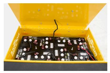
Figure 10: The battery compartment of the PMT-4500 NGX is located under the seat. To access the battery compartment, grasp the back of the seat and push it forward. The batteries are connected in series, as shown in the diagram in Figure 11.
