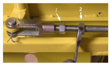
Figure 13 The brake rod showing the (1) jam nut and (2) adjustment nut. The jam nut must be loosened before the brake rod is adjusted and retightened after the adjustment. Each of the two brake rods, one on either side, should be adjusted equally.
