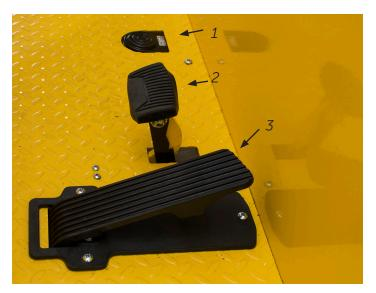
Figure 6: The floor of the operator area, showing (1) the accelerator/brake pedal, (2) the parking brake, and (3) the left-foot presence switch. With the key switch turned to "On", and the directional switch at "Forward" or "Reverse," and the left foot on the left-foot presence switch, pressing the pedal puts the vehicle in motion. When the pedal is released, the vehicle stops.
