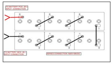
Figure 11: The batteries connected in series.
