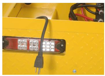
Figure 3: The AC cord is stored in the engine compartment. To charge the battery, make certain that the AC cord is connected to the charger cord and to a dedicated 120 V. outlet.
