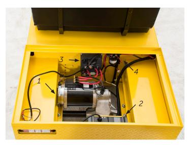
Figure 9: The motor compartment is accessed by removing the cargo deck. The parts of the motor system shown above are (1) the AC motor, (2) the on-board battery charger. (3) the controller, and (4) the 10-amp fuse. The fuse should always be removed before performing any maintenance or repair work on the vehicle.
