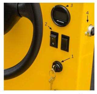
Figure 4: The instrument panel showing (1) the on/off switch, (2) the directional selector switch, (3) the Smart View display and (4) the horn..
