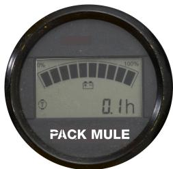
Figure 5: The Smart View display is standard on all Pack Mule vehicles. The top of the display shows the battery state of charge, the numbers indicate the traction hours. If there is a fault, the fault code is displayed in the bottom part of the display. An explanation of the fault codes begins on page 16.
