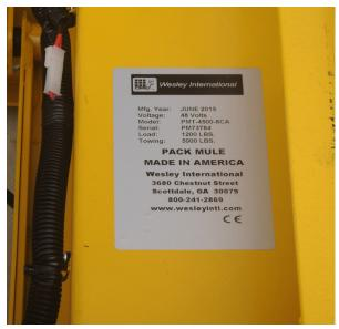
Figure 2: The Vehicle Identification Plate is located on the inside of the motor compartment. Please refer to this information when requesting warranty service, ordering replacement parts, or requesting service support from Wesley International.
