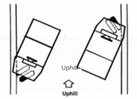
Figure 8: Proper positioning of the Pack Mule's front wheels when parking on an incline.
