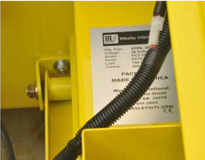
Figure 2: The Vehicle Identification Plate is located on the inside of the motor compartment. Please refer to this information when requesting warranty service, ordering replacement parts, or requesting service support from Wesley International.
