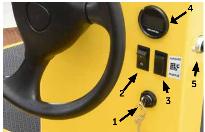
Figure 5: The instrument panel showing (1) the key switch, (2) the rocker on/off switch, (3) the directional selector switch, (4) the Smart View display, and (5) the horn button..
